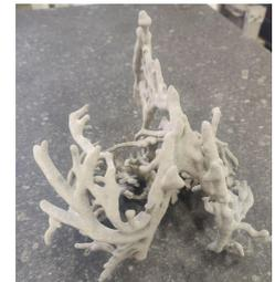
3D printed vascular model of a Rat's Brain.
